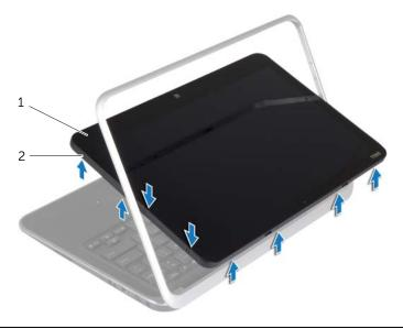
display panel screws (8) **3** Rotate the display and remove the screws that secure the display back-cover to the display panel.
